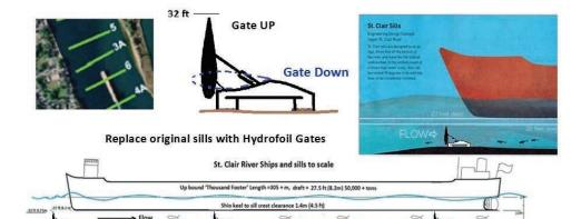
USACE Type 4 Sills replaced by hydrofoil gates in sections on original footprint
